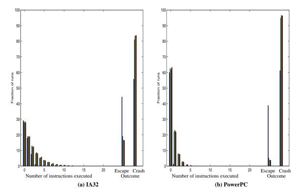
Fig. 4. Proportion of runs that fail after exactly n instructions, with memory density 0.05, for (a) IA32 and (b) PowerPC. On the right, the proportion of escaped vs. crashed runs is presented for comparison. Each instruction length bar is composed by five sub-bars, one for each random block (simulated attack) sizes 4, 16, 28, 40 and 52 bytes, left to right.
