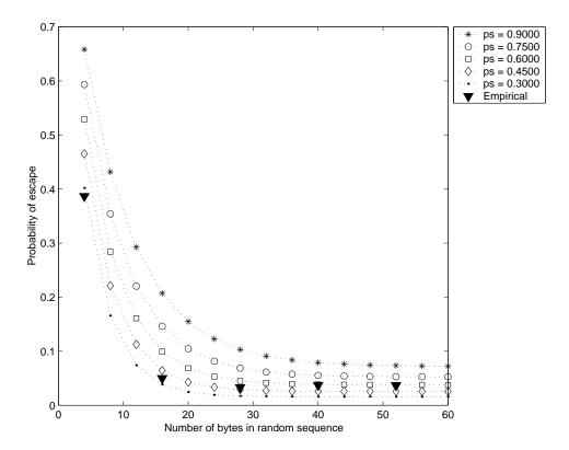
Fig. 6. Theoretical probability of escape for a random string of n symbols. Each curve plots a different probability of executing a process-state-determined memory access  $(p_s)$  for the PowerPC uniform-length instruction set. Process memory occupancy is fixed at 0.05. The large triangles are the measured data points for the given memory occupancy (data taken from Figure 3 for the PowerPC and memory density q=0.05), and the dotted lines are the predicted probabilities of escape.
