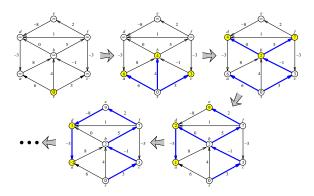
Four phases of Moore's algorithm run on a directed graph with negative edges.
