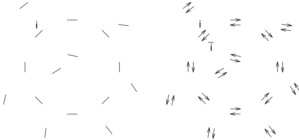
Figure 1: Left: An input pattern consisting of N edges. Each edge, i , has a position, \vec{x}_i , and an orientation, \theta_i . Right: A set of 2N states, S . For each edge, i , in the input pattern, there are two states, i and \bar{i} , in S . The two states associated with an edge have the same position, but are opposite in direction. That is, \vec{x}_i = \vec{x}_{\bar{i}} but \theta_i = \theta_{\bar{i}} + \pi . These two states represent the two possible directions a particle undergoing a random motion can visit an edge of the input pattern.
