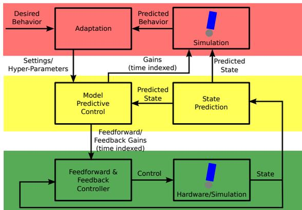
Fig. 1. Structure of our adaptive, real-time motion control framework. A standard full-state feedback controller (green) is complemented with an optimization-based, model predictive controller (yellow). Through an additional adaptation layer (red) higher-level behaviors can be specified.
