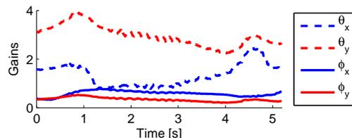
Fig. 5. Evolution of tilt angle and ball rotation angle feedback gains during a go-to task. The slowly varying gains validate the smooth behavior that the MPC structure generates.
