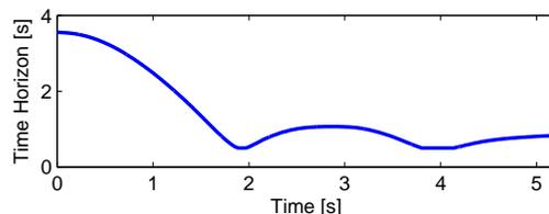
Fig. 4. Scaling of the time horizon for the finite time optimal control algorithm (iLQG). While approaching the goal, it is reduced (limited to a lower boundary of 0.5 s) to ensure a good position tracking.
