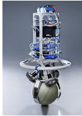
Fig. 2. Photograph of the ball balancing robot Rezero which is used during our experiments for validating the performance of the proposed approach. Due to its static instability and non-minimal phase behavior, it poses interesting challenges in terms of dynamics to the control approach. Photo: Gerhard Born, Ringier AG
