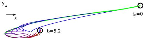
Fig. 3. Overhead plot of continuously recomputed, predicted MPC paths (blue to red gradient) and the executed path (green) of a go-to task on Rezero. The time horizon is adapted online based on the goal distance.
