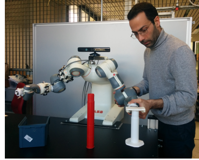
Fig. 1. Demonstrating the manipulation example with ABB FRIDA prototype (YuMi). A cylinder is considered as an obstacle on the table during demonstration.
