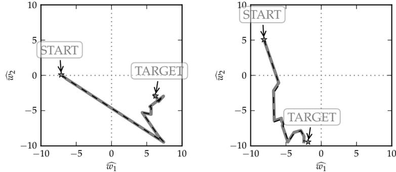
**Fig. 5.** Two example weight traces from DNA learning circuit simulations (grey solid lines), overlaid with corresponding traces from our Python reference implementation (black broken lines). The lines coincide closely in all simulations, not just the examples shown here, indicating that the DNA circuit works correctly.
