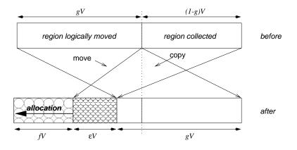
Figure 8: Operation of the oldest-first collector.
