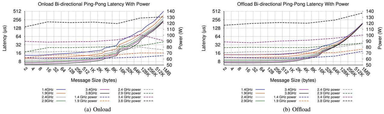
Fig. 5: Onloaded vs. offloaded bi-directional ping-pong latency
