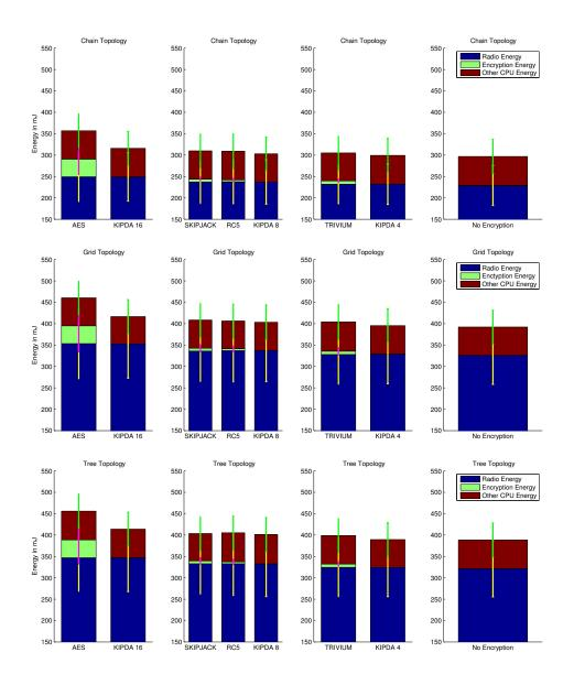
Figure 5.9: Average energy used per node in a WSN using KIPDA MAX/MIN aggregation and hop-by-hop aggregation using AES, SkipJack, RC5, and Trivium encryption for three topologies from Figure 5.7. 333 Aggregations were performed. The number after KIPDA indicates the number of bytes for a message vector.
