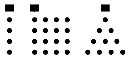
Figure 5.7: Example of three different topologies: chain, grid, and tree, used to test KIPDA against hop-by-hop encryption. Squares represent the base stations and circles represent the nodes. 49 nodes were used in all simulations.
