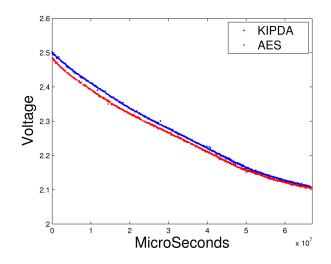
Figure 5.13: Comparison of voltage used between KIPDA with a message vector of 18 bytes, and hop-by-hop aggregation with the AES cipher that used 16 byte blocks. Comparisons took place on Moteiv T-mote Invent (TelosB architecture) sensors.
