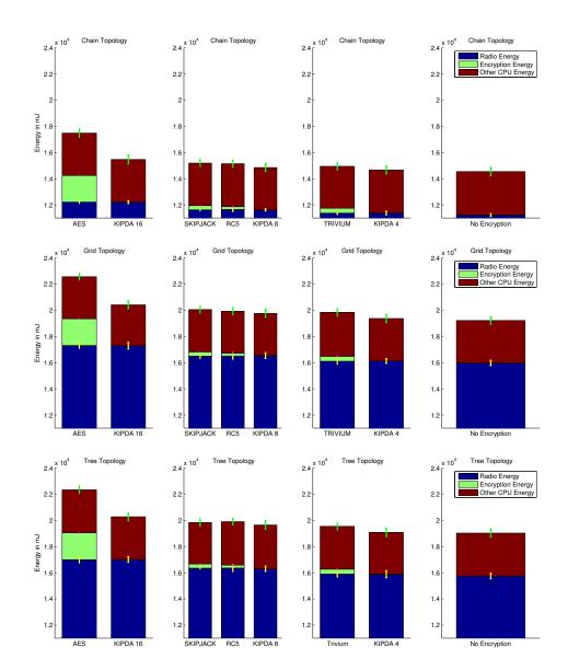
Figure 5.8: Total energy consumption for a WSN of 49 nodes using KIPDA MAX/MIN aggregation and hop-by-hop aggregation using AES, SkipJack, RC5 and Trivium encryption for three topologies from Figure 5.7. 333 Aggregations were performed. The number after KIPDA indicates the number of bytes for a message vector.
