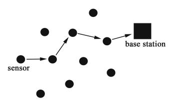
Figure 2.1: Example of a wireless sensor network. Because of the limited radio range of the sensor nodes, they route information through each other to reach a base station.
