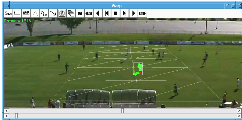
(a) Soccer footage from a single camera, 720 x 240 pixels. The system is tracking a single player. The player's estimated position is the red dot.
