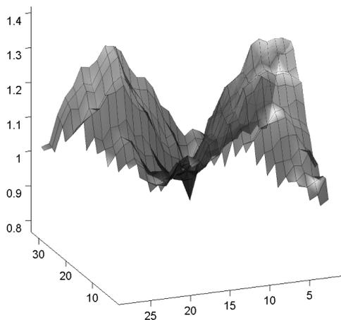
Figure 3:  $C(M)/C(\mathcal{M}_{total})$  for bone contours as function of split positions if split into two sub-shapes. Note the deep minimum (0.841) at the correct split position.
