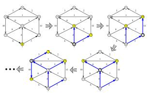
Four phases of Dijkstra's algorithm run on a graph with no negative edges. At each phase, the shaded vertices are in the heap, and the bold vertex has just been scanned.
