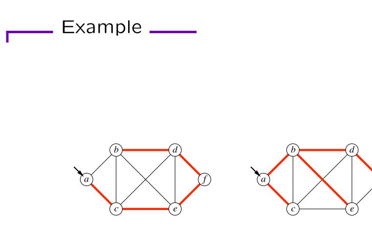
A depth-first spanning tree and a breadth-first spanning tree of one component of the example graph, with start vertex a.
