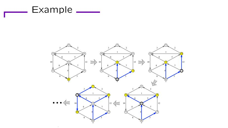
Four phases of Dijkstra's algorithm run on a graph with no negative edges. At each phase, the shaded vertices are in the heap, and the bold vertex has just been scanned.
