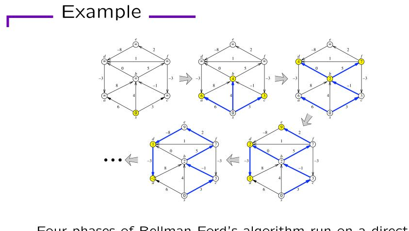
Four phases of Bellman-Ford's algorithm run on a directed graph with negative edges.
