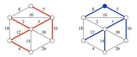
A minimum spanning tree (left) and a shortest path tree rooted at the topmost vertex (right).
