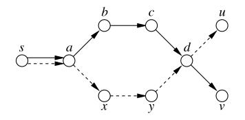
If  $s\to a\to b\to c\to d\to v$  and  $s\to a\to x\to y\to d\to u$  are both shortest paths,
