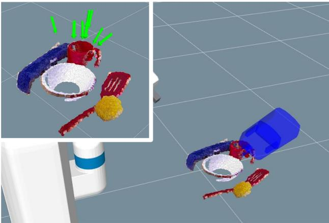
Fig. 3: Grasp calculation and preference data selection. (Top) Selecting a segmented object to grasp in the GUI. (Bottom) Grasp Selection Window with green arrows shown in the corner of the main window. The main window shows the currently selected grasp.
