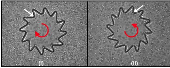
Fig. 3. Collisions between swimming bacteria in solution and micro-gear boundaries result in unidirectional rotation of the microstructure (i) Clockwise rotation direction observed for micro-gears exhibiting counterclockwise oriented teeth (ii) Counterclockwise rotation direction observed for micro-gears exhibiting clockwise oriented teeth
