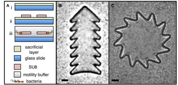
Fig. 1. (A) MBR microfabrication and design. (i) Glass slide spin coated with dextran (ii) SU8 patterning via photolithography (iii) MBRs release in a semi-dilute suspension of swimming bacteria and bacteria collide with walls. (B) Micro-chevron with boundary comprised of 14 teeth. (C) Micro-gear with boundary comprised of 12 teeth. Each scale bar is  $15\mu\text{m}$
