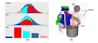
Fig. 2. (a) Distribution of the features according to the classes in the generated model. From bottom to top: number of instances for each of the classes; distribution of the data by time; distribution of data by distances, in color the number of instances assigned to each class is shown; (b) trajectories used for simulation experiments, which are generated for PR2 unhang and putdown wheel actions in OpenRave.
