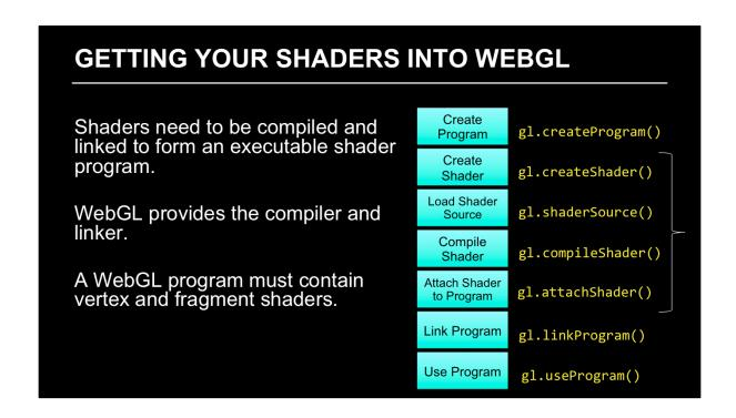
Shaders need to be compiled before they can be used in your program. As compared to C programs, the compiler and linker are implemented within WebGL, and accessible through function calls from within your program. The diagram illustrates the steps required to compile and link each type of shader into your shader program. A program must contain a vertex shader (which replaces the fixed-function vertex processing), a fragment shader (which replaces the fragment coloring stages).
