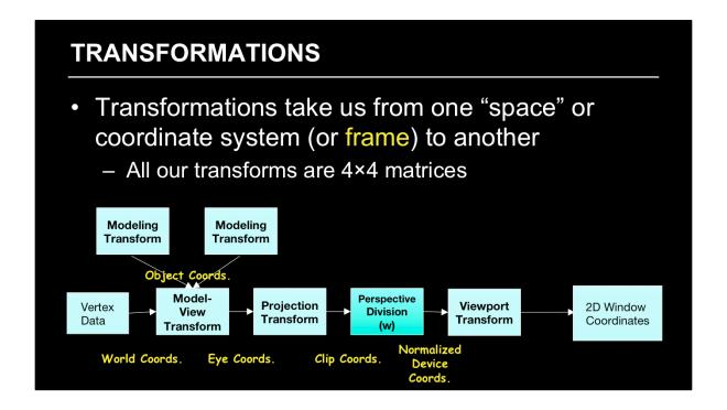
The processing required for converting a vertex from 3D or 4D space into a 2D window coordinate is done by the transform stage of the graphics pipeline. The operations in that stage are illustrated above. Each box represent a matrix multiplication operation. In graphics, all our matrices are 4×4 matrices (they're homogenous, hence the reason for homogenous coordinates).
