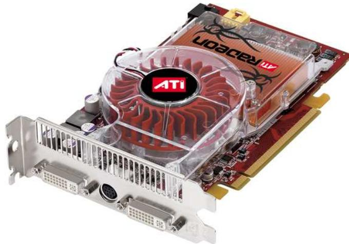
Figure 2.6: ATI Radeon X850 board (graphics card)
