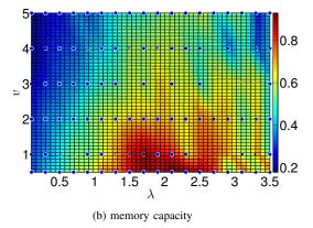
Fig. 2: (a) Examples of node dynamics in the reservoir (left columns) and corresponding power-spectral density (PSD) (right column). The existence of power-law PSD indicates non-trivial long-term memory at the level of single nodes similar to what was reported in [9]. (b) Memory capacity C as a function of input weight coefficient v and spectral radius  $\lambda$ . The values are normalized by system size N=20.
