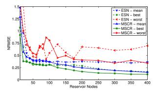
Fig. 4: NARMA performance for increasing SCR sizes. The dashed lines are obtained with regular sigmoidal neurons (ESN) and v=0.01 and  $\lambda=0.75$ . The memristive SCR (MSCR) data was obtained based on v=0.5.  $\lambda=1.7$ , and 52 memristive devices on average per node.
