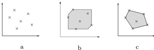
Figure 2: (a) A set of points in 2D and its approximation using a (b) zone and (c) polygon region.
