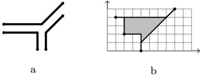
Figure 3: (a) Three possible shapes of a max-plus line segment:  $\max(x + a, b) \geq y$  (top),  $\max(y + a, b) \geq x$  (right),  $\max(x + a, y + b) \geq 0$  (left) and (b) a max-plus convex hull built over four points using these line segments.
