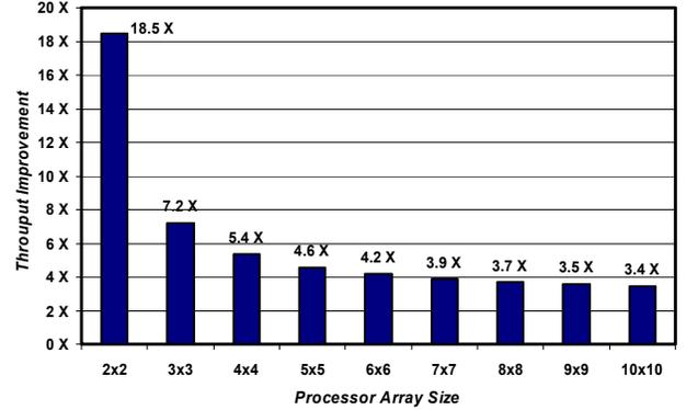
Figure 5. Predicted maximum throughput improvement in HNoC versus conventional NoC for different array sizes, assuming that  $p=0.6$
