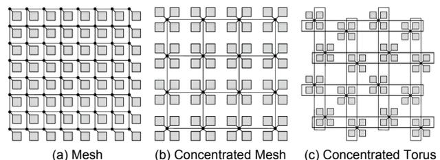
Figure 1. Three examples of NoC topologies [3].
