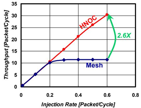
Figure 7. Simulation results for HNoC throughput
