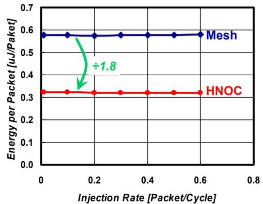
Figure 8. Simulation results for HNoC energy per packet
