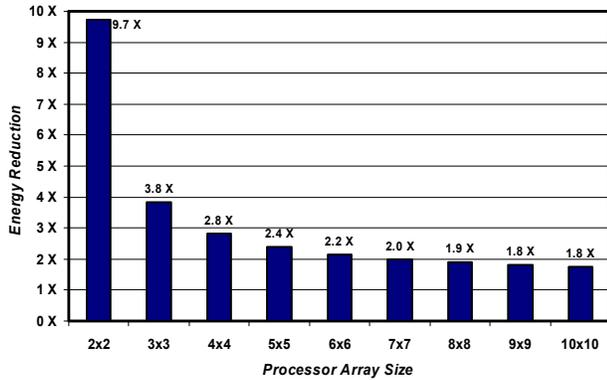
Figure 6. Energy reduction in HNoC compared to conventional NoC for different array sizes when  $p=0.6$
