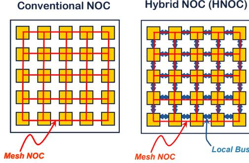
Figure 2. HNoC versus conventional NoC
