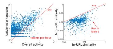
**Fig. 6.** Comparing the normal activity of a user with its activity near the handovers. 97.4% of the users have higher activity-per-hour around handovers. Both x-axis and y-axis are in log scale. (right) The plot shows how the content of the tweets changes with URL changes.
