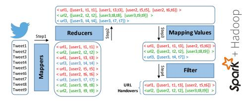
**Fig. 4.** The process of detecting URL handovers in the Twitter network. 2 URL handovers are detected from 9 tweet objects in this example.
