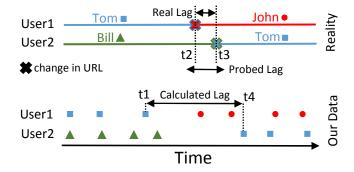
**Fig. 3.**  $User_1$  handed over the URL Tom to  $User_2$ . The release time is  $t_2$  and the claim time is  $t_3$ , and the real handover lag is  $t_3 - t_2$ . We calculate an upper bound,  $t_4 - t_1$ , for the handover lag based on the last tweet of  $User_1$  at  $t_1$  before the handover, and the first tweet from  $User_2$  at  $t_4$  after the handover.
