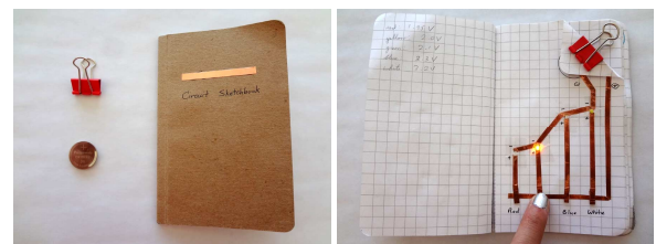
Figure 7. Standard sketchbook with coin cell and binder clip power supply. Example page.
