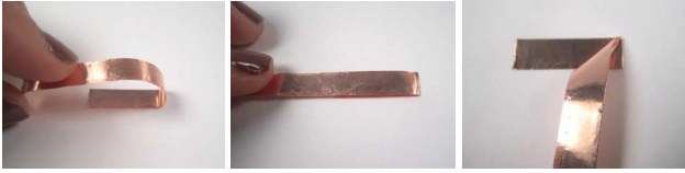
Figure 2. Making sharp turns: (a) Fold the foil tape back on itself, (b) so the sticky side faces up. (c) flip it over while simultaneously folding the corner and flatten.
