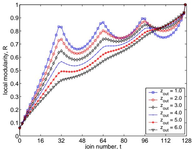
FIG. 2: Local modularity  $R$  as a function of the number of steps  $t$ , averaged over 500 computer-generated networks as described in the text; error bars are omitted for clarity. By varying the expected number of inter-community edges per node  $z_{out}$ , the strength of the community boundaries are varied.
