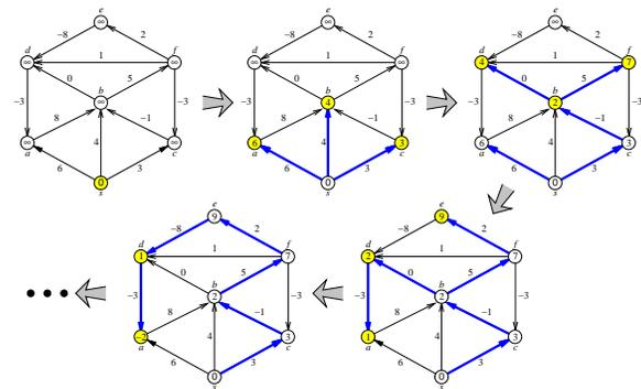
Four phases of the Bellman-Ford algorithm run on a directed graph with negative edges.
