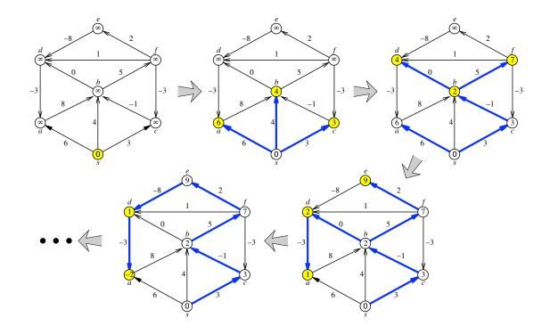
Four phases of Bellman-Ford's algorithm run on a directed graph with negative edges.
