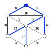
A minimum spanning tree (left) and a shortest path tree rooted at the topmost vertex (right).
