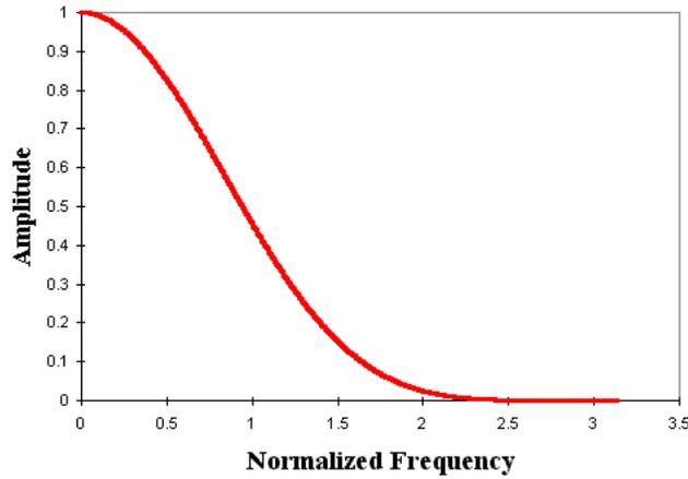
Figure 2.3: Recursion low-pass filter  $L_1$  for original shiftable pyramid.
