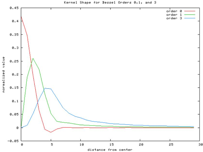
Figure 3.8: Radial kernel profile as function of angular function order.
