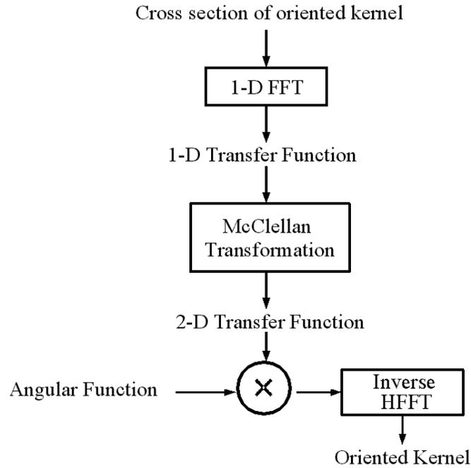
Figure 3.9: Procedure for constructing an oriented kernel by resampling method.
