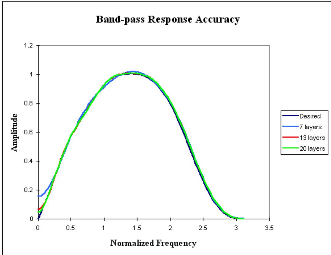
Figure 4.2: Band-pass responses for 7, 13, and 20 hexagonal kernel layers.
