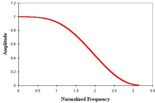
Figure 2.6: Initial low-pass filter  $L_0$  for standard shiftable pyramid.
