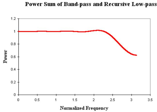
Figure 2.10: Power sum of band-pass and recursion low-pass filters.
