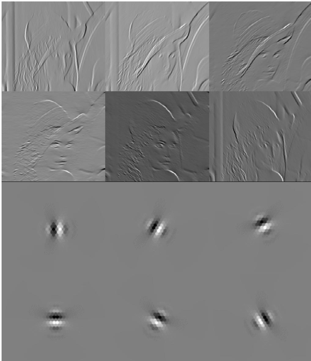
Figure 4.4: “lena” image convolved with six  $\cos^5(\theta)$  basis kernels.
