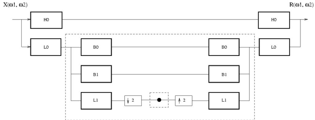
Figure 2.1: Block diagram of pyramid decomposition
