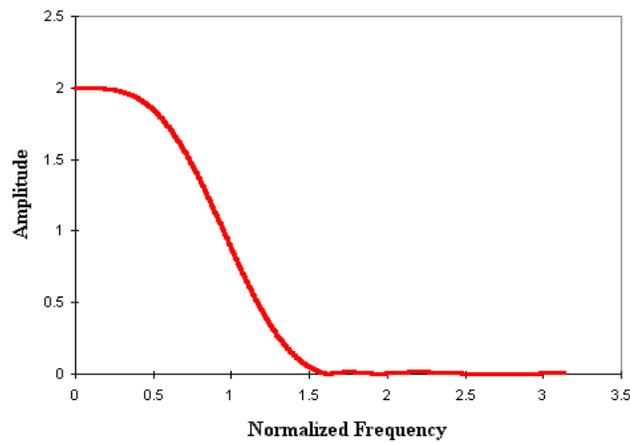
Figure 2.7: Recursion low-pass filter  $L_1$  for standard shiftable pyramid.
