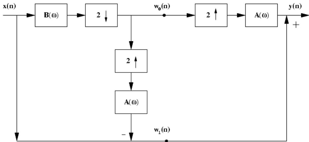
Figure 1.2: Laplacian pyramid block diagram
