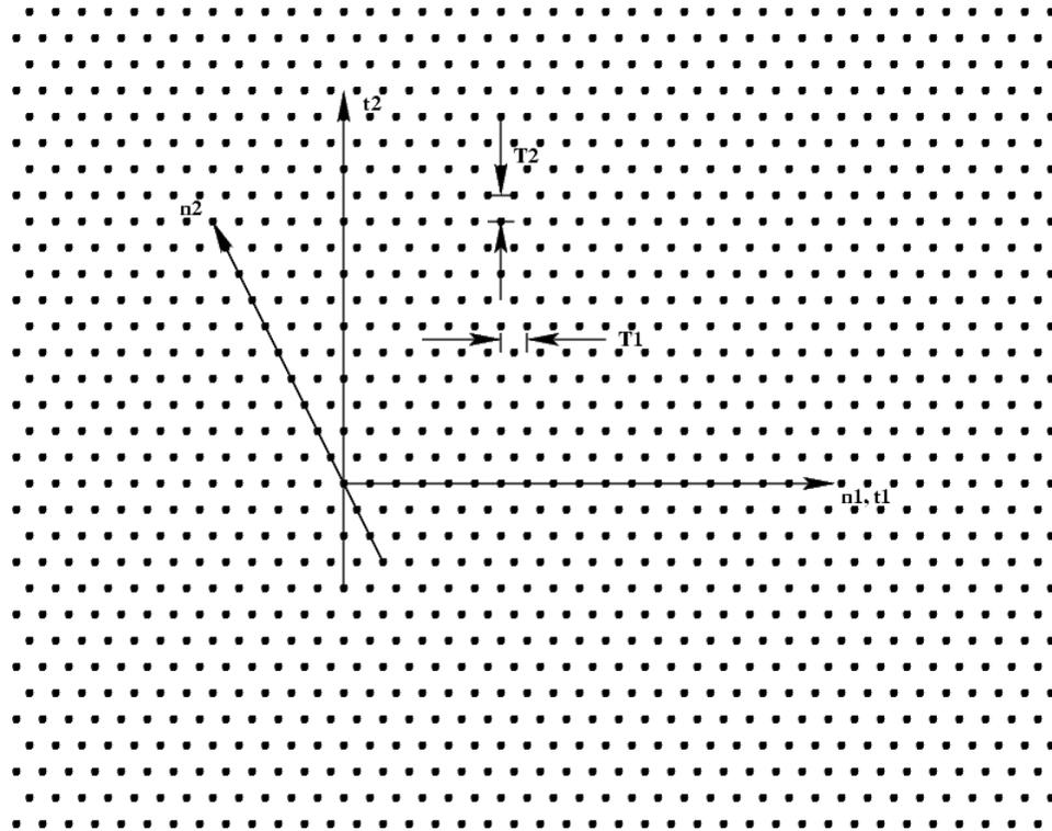
Figure 3.3: Grid and coordinate system for hexagonal sampling
