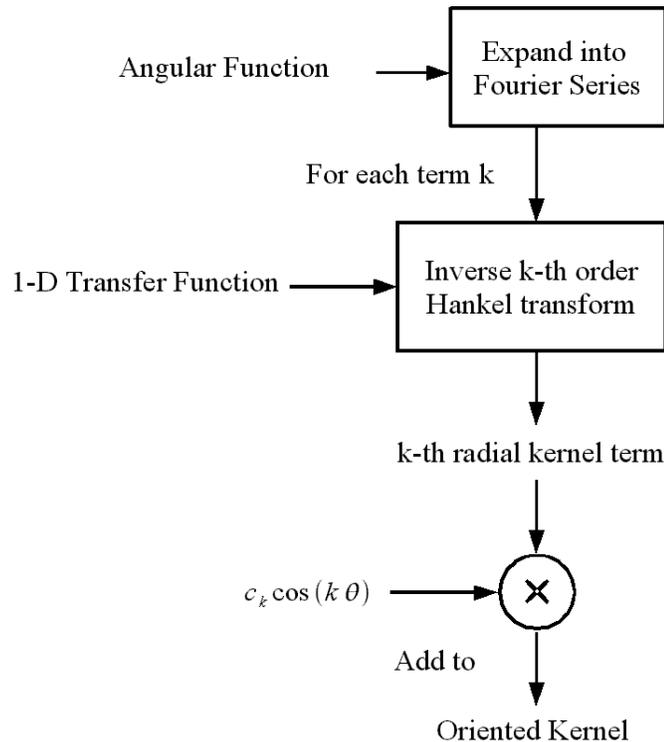
Figure 3.7: Procedure for constructing an oriented kernel by analytical inverse polar Fourier transform.
