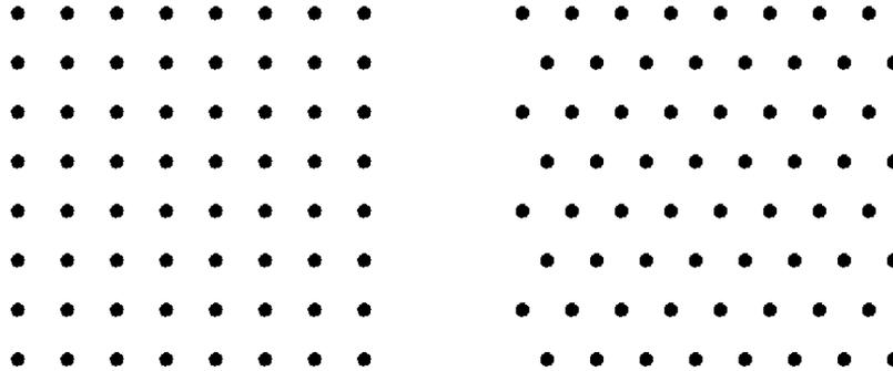
Figure 5.1: Square and hexagonal downsampling patterns for noise reduction comparison.
