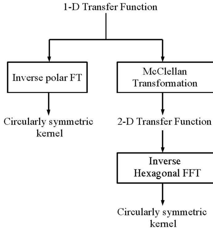
Figure 3.1: Two kernel construction methods for circular filters.
