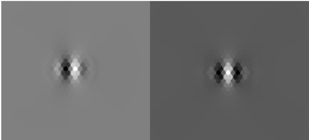
Figure 5.2:  $0^\circ$  basis kernel for  $\cos^5(\theta)$  oriented filter and its quadrature counterpart.
