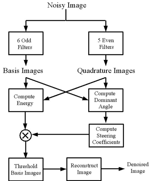
Figure 5.7: Noise reduction by local orientation analysis.
