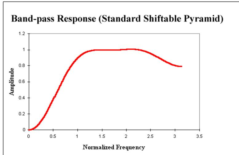
Figure 2.8: Band-pass filter  $B$  for standard shiftable pyramid.
