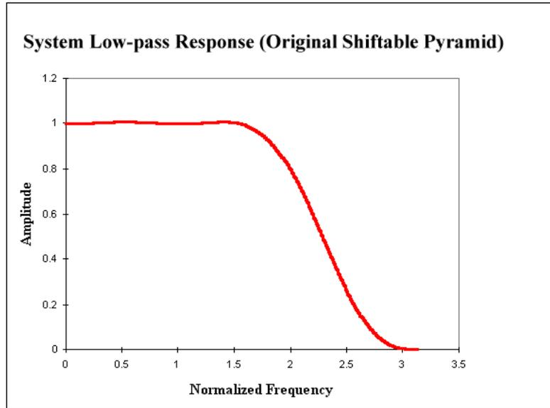
Figure 2.2: Initial low-pass filter  $L_0$  for original shiftable pyramid.
